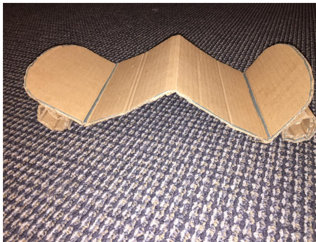
Figure 6: The triple fold skateboard reveals the flaws associated with having too many points of folding in any of our designs.
