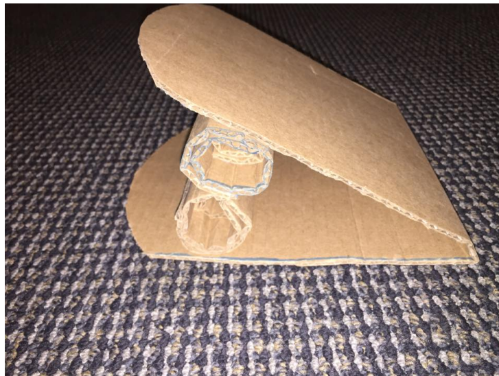
Figure 4: The classic fold skateboard uses the most obvious method of folding a skateboard down its horizontal center to reduce size.
