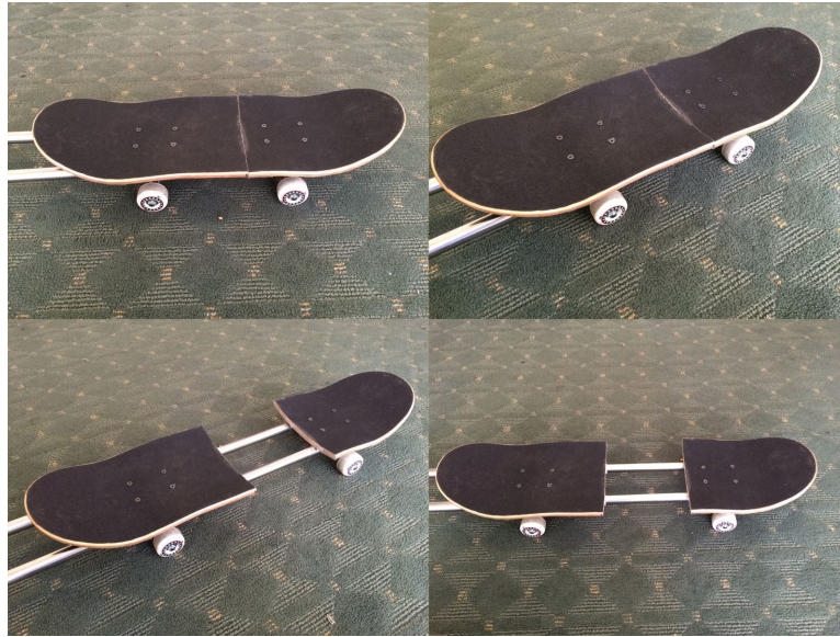
Figure 13: Our team’s first “rideable” Pocket Board , featuring both expandability and concealability by fitting into a conventional backpack.
